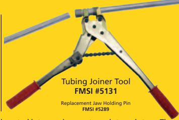
During assembly of a connection, the tubes to be joined are inserted into a union, up to an internal stop. The assembly tool (FMSI #5131) is then used to apply pressure to the union, which compresses to complete the connection. This is a quick and simple method of joining tubes that eliminates the fire hazards of brazing and proper torque concerns of threaded connections, while producing permanent leak-free connections.
