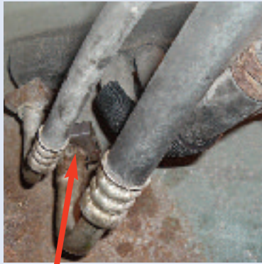
Leaking refrigerant lines at spring lock connection.
